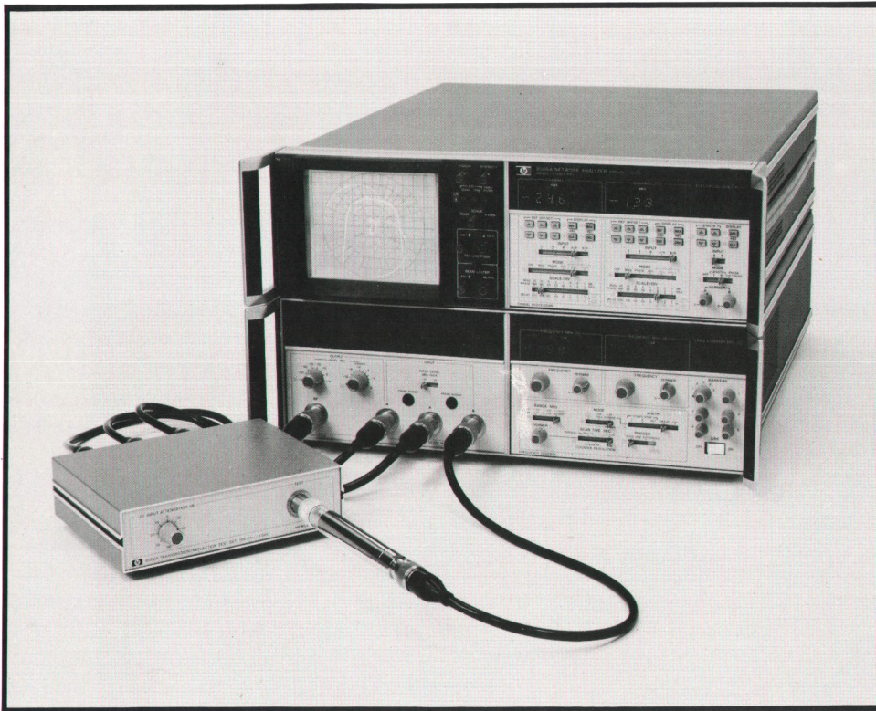
Fig. 1. Model 8505A Network Analyzer is shown here measuring the transmission and reflection coefficients of a 50 \Omega filter using the Model 8502A Transmission/Reflection Test Set. With its digital readouts, in addition to a dual-mode CRT display, this new instrument can characterize circuits and components in the 0.5 - 1300-MHz frequency range more quickly, more accurately, and with greater convenience and less ambiguity than its predecessors.
