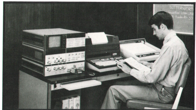
Fig. 5. Factory-assembled and tested automatic systems designed around the Model 8505A Network Analyzer are furnished with example programs and programs for accuracy enhancement, system verification, and diagnostic testing.
